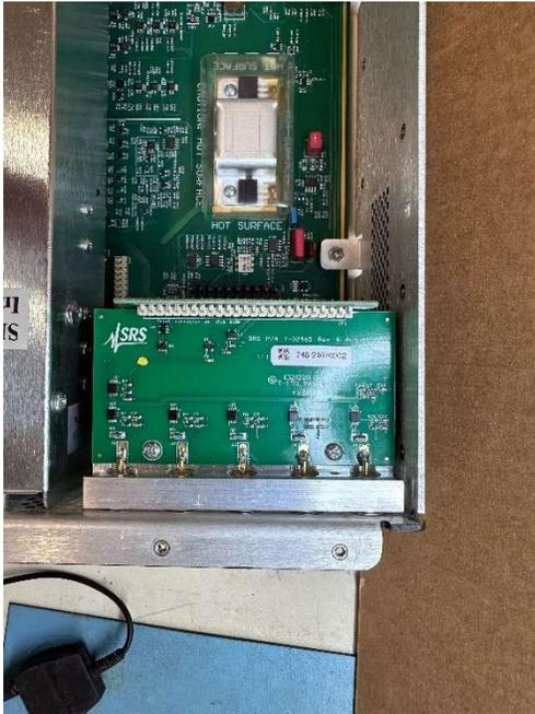
4. Lastly, secure the assembly with the screws provided (see picture below).
