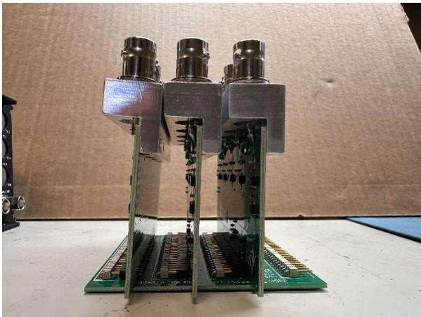
3. Now install the assembly into the FS740 so the BNC connectors on the option card(s) fit through the holes in the back of the instrument. Once the assembly is in place, seat the multi-pin connector into the mating connector on the motherboard of the FS740.
